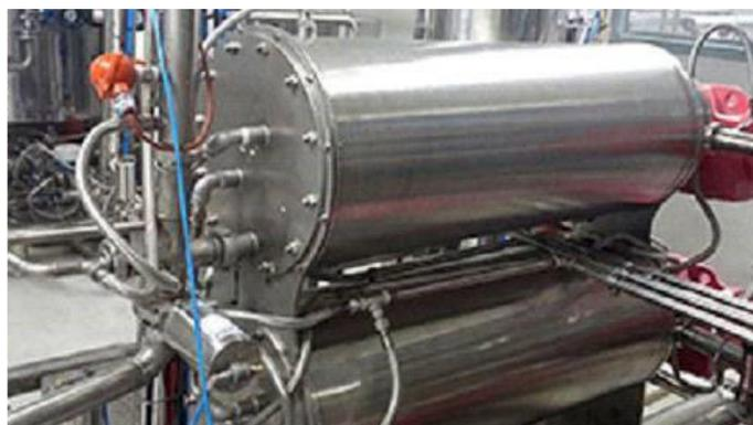
Mixing and aeration tanks where the product is mixed with air
